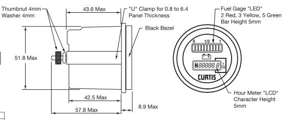
Note: In addition to a "U" clamp and thumbnuts/washers shown in the drawing, individually packed units are provided with a mating connector and female pins. Bulk packed units are provided with a "U" clamp and hex nuts/washers only.
