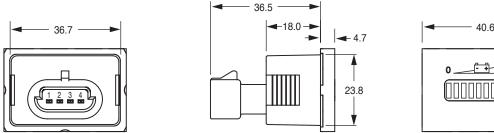
NOTE: Equivalent to Delphi-Packard connector P/N 15336035 4-pin.
